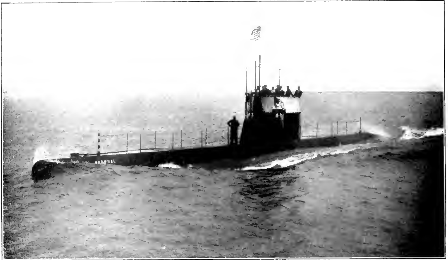
THE LATEST TYPE OF AMERICAN SEA-GOING SUBMARINE THE U. S. S. "NARWHAL," WHICH CAN GO 150 MILES UNDER WATER AT A SPEED OF 11 KNOTS AN HOUR, AND MUCH FARTHER ON THE SURFACE WITH A MAXIMUM SPEED OF 14 KNOTS
